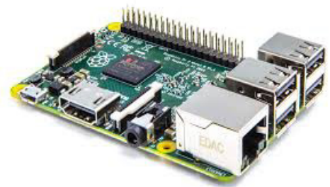
Raspberry Pi computer - costs $37 and is the size of a credit card
